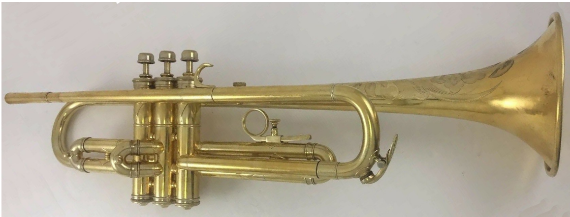
#95323 Revelation c.1927 (auction) showing the new design with the first valve slide branches vertical rather than offset
